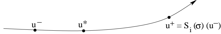
Figure 16: The i -shock (u^-, u^+) satisfies the Liu admissibility conditions if its speed satisfies \lambda_i(u^-, u^+) \leq \lambda_i(u^-, u^*) for every intermediate state u^* along the i -shock curve through u^- .
